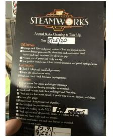
H2 — Steam boilers require regular maintenance and this label shows the most recent service was on 8/25/20. 82.9% efficiency is acceptable for equipment of this type and age but newer boilers can reach 97%.
