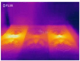
Photo E-17 – This infrared photo of the Metcalf kitchen range shows the pilot lights are burning  $24 \times 7$ .
