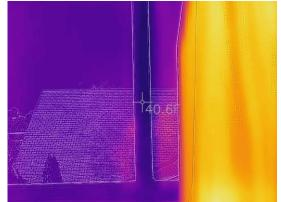
BE-21 -- Infrared photo shows poor thermal performance of single pane aluminum frame windows.
