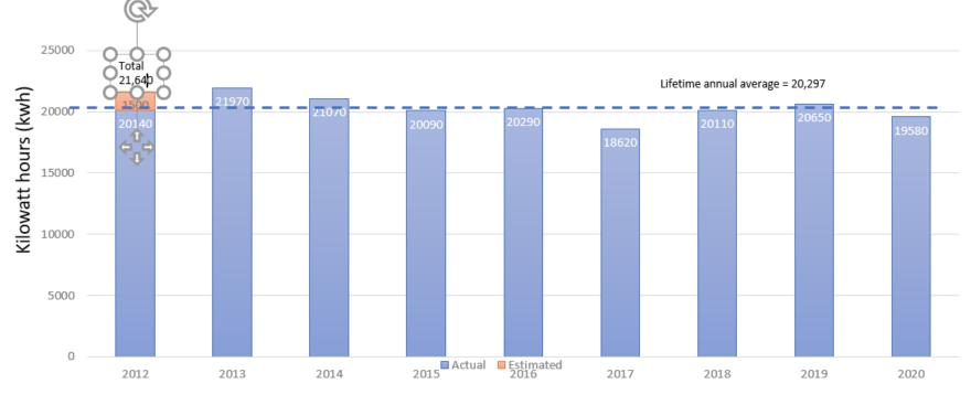
Note that in 2012 – 2014, production was over 21,000 kwh, then dropped to 20,000 in 2015 and has stayed there. It is possible that one or more panels or microinverters has malfunctioned. Pegasus is responsible for the repair and maintenance of the system and should perform a system check.
